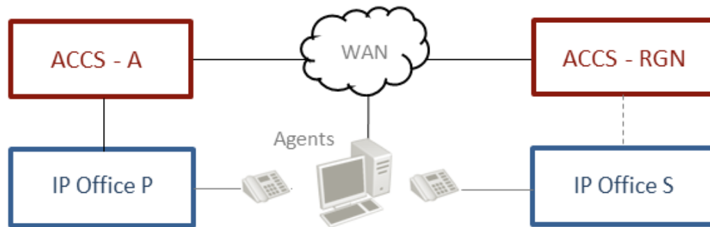
Figure 6: A diagram depicting an Avaya Contact Center Select Geographic Business Continuity solution in which the ACCS active server connects to an IP Office primary server in an IP Office resilient system
