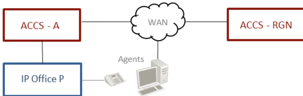
Figure 5: A diagram depicting an Avaya Contact Center Select Geographic Business Continuity solution in which the ACCS active server connects to an IP Office server
